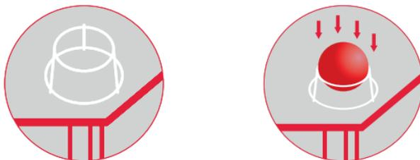
For placement in manual mode, the universal mount is used as a stand, which is located with a large diameter of the mounting circle down.
