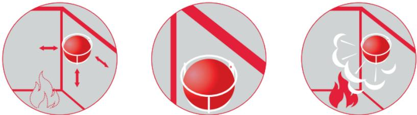
1. Place the device at a distance of up to 30 cm from the top or side above the place of high risk of fire.
