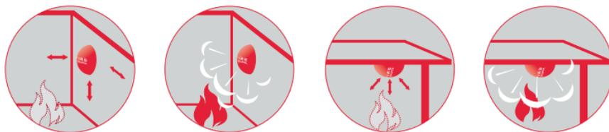
1. Place the device at a distance of up to 30 cm from the top or side above the place of high risk of fire.
