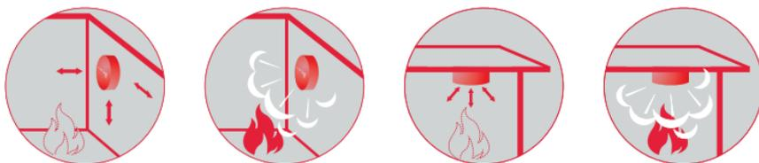
1. Place the device at a distance of up to 30 cm from the top or side above the place of high risk of fire.
